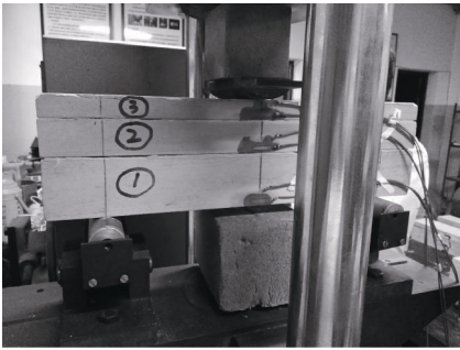
图 2 简化模型抗弯试验装置 Fig.2 Bending resistance test device for simplified model
