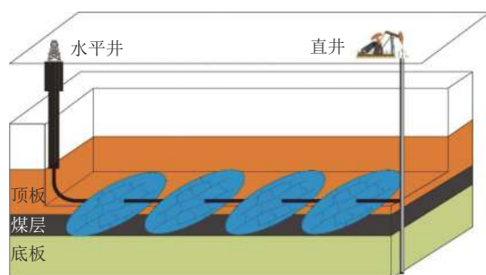
图1 煤层顶板分段压裂水平井技术原理 Fig.1 Schematic diagram of the staged fracturing horizontal well in coal seam roof
